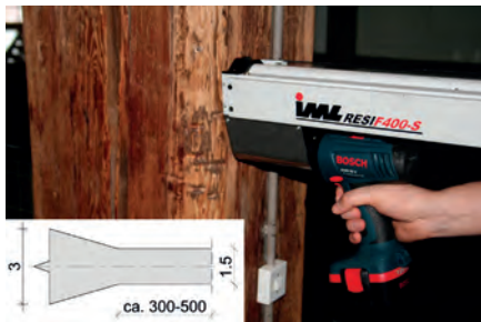
Rys. 2. DRM system dostosowany do badania drewna Fig. 2. Resistance drilling system adopted for testing timber structures
